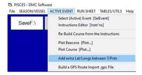
This option is used when the GPS device TTG/TTN (Time to Go/Time to Next) method is used. Note that the GPS speed is used to calculate the time.
